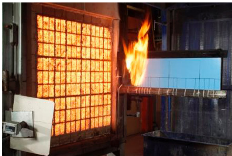
Figure 9 - BS 476 Part 7 test apparatus
